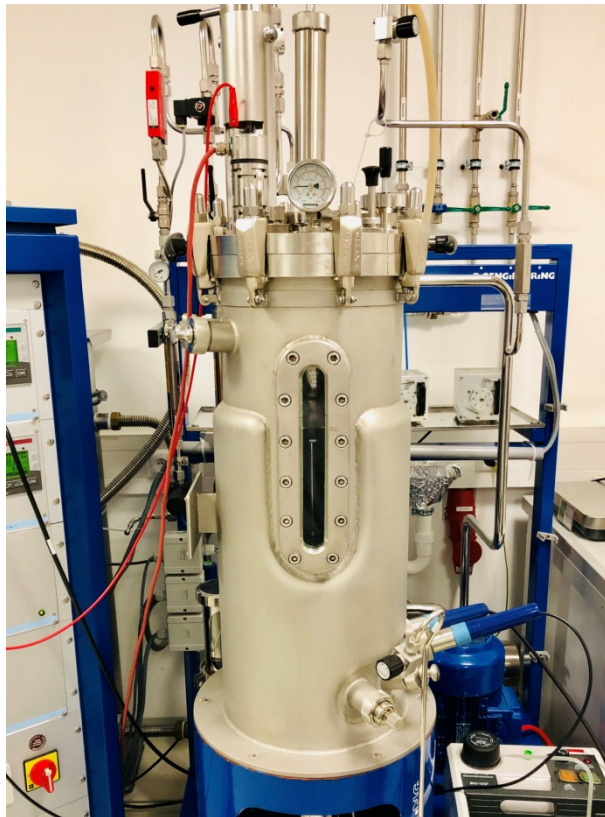
Fig. 2. Reactor holding cell culture for manufacturing recombinant proteins such as Factor C.
